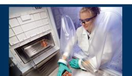
Cells are totally isolated in closed system. No bunny suits required.
