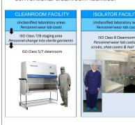
The isolator is certified to ISO Class 5 and is housed within an ISO Class 8 cleanroom\*. These are the air cleanliness classifications required for isolator facilities engaged in the aseptic manufacture of human therapeutic products
